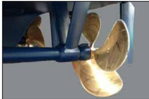
*Enclosed propeller shaft and rope cutter*
