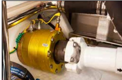
*Sea Torque thrust assembly*
